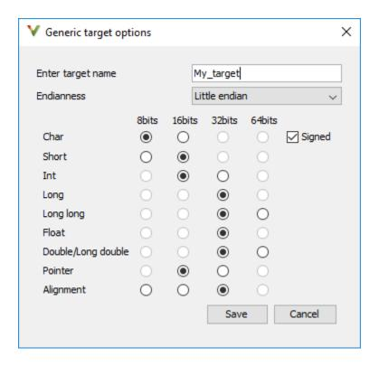
Use the dialog box to specify the name of a new mcpu target, for example My\_target. That new target is added to the **Target processor type** option list.
